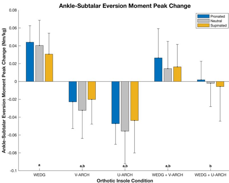
**Fig. 4.** Change in peak ankle/subtalar eversion moment compared to FLAT. **a** and **b** along the x-axis denotes a significant difference between the insole condition and FLAT and WEDG, respectively ( $p < 0.05$ ). Please note that since calculated negative values for ankle/subtalar frontal plane moments refer to the eversion direction (see Appendix 1), more negative values (higher eversion moments) for a given condition are depicted as positive amounts in this eversion moment change graph.
