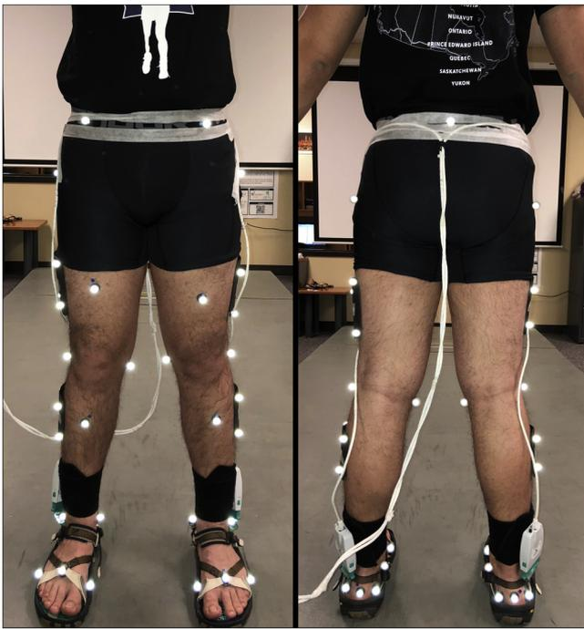
Fig. 2. Marker set-up used during static calibration trial.
